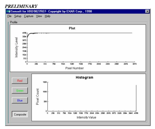
Figure 11. White Target Scan After Gain Adjustment
